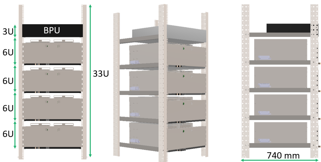
Figure 10: Rack design of the Solitek module from a different perspective
